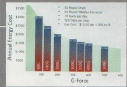
finisher without slowing down the productivity. The high speed or G-force is the driving factor. By utilizing the inverter technology it has been possible to achieve this high-speed extraction in freestanding machines. The inverter is automatically measures the out of balance electronically and decides if the machine can proceed to high speed generating the high G-force.
